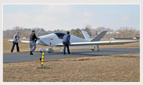
With only a crew of four, the Teros can complete many of the same missions that usually require a crew of 20 or more. Despite being a large UAS airframe, Teros is designed for trailer transport with easily removable wings.
